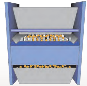
Material released from the gated Universal Splitter Hopper flows evenly across the entire width of the chutes.
