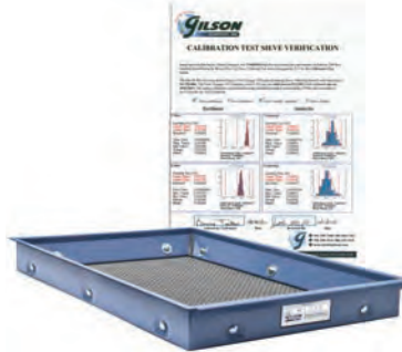
GV-66 Calibration Verification shown with Screen Tray
